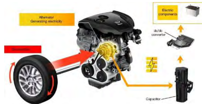
Figure 20: Super capacitor integrated automotive regenerative braking system overview
