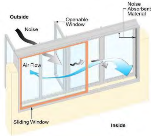
Figure 2: Schematic diagram showing the working mechanism of acoustic window (baffle type)
