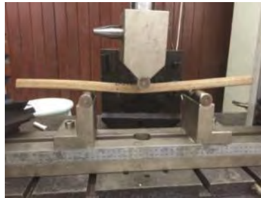
Figure 1115: Bending test -shear modulus via variable span method (Author)
