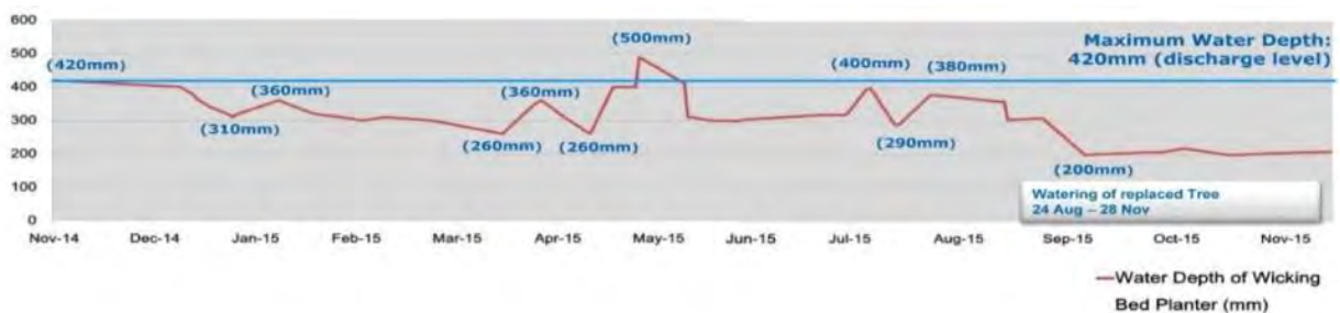
Figure 10: Records of water level of ZIS at Homantin Site
