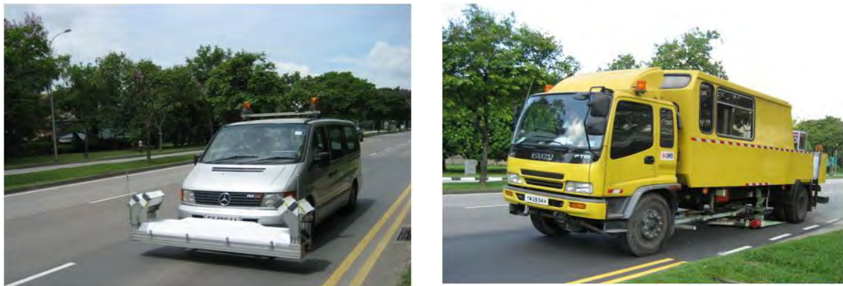
Figure 2: Left: laser profiler; right: deflectograph
