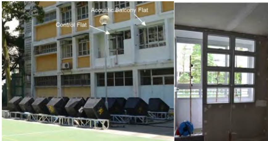
Figure 8: Mock-up flats for comparison of the performance of enhanced acoustic balcony and conventional window
