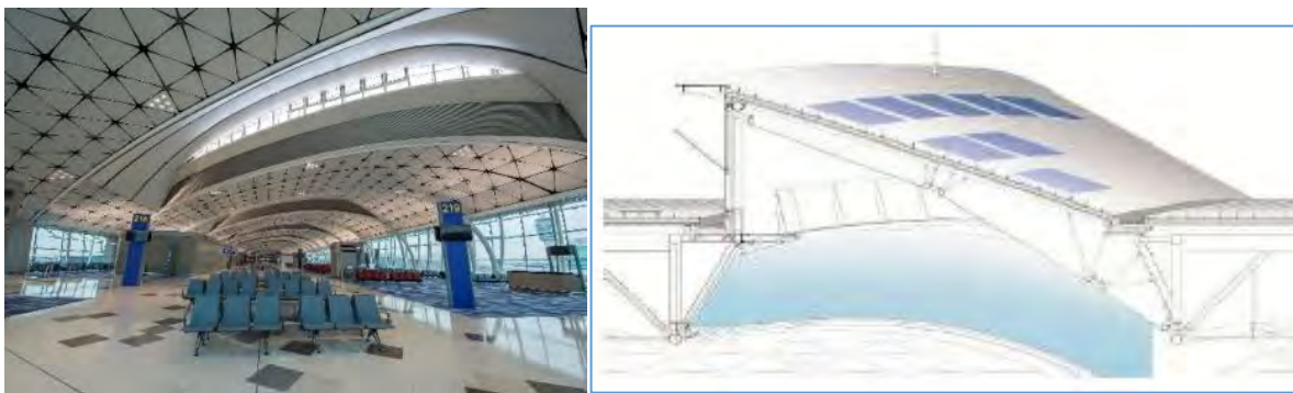
Figure 3: Design of north-facing skylights located on roof along the true east west axis of MFC
