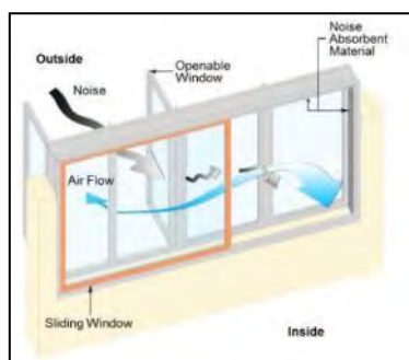
Figure 3: Configuration of acoustic window
