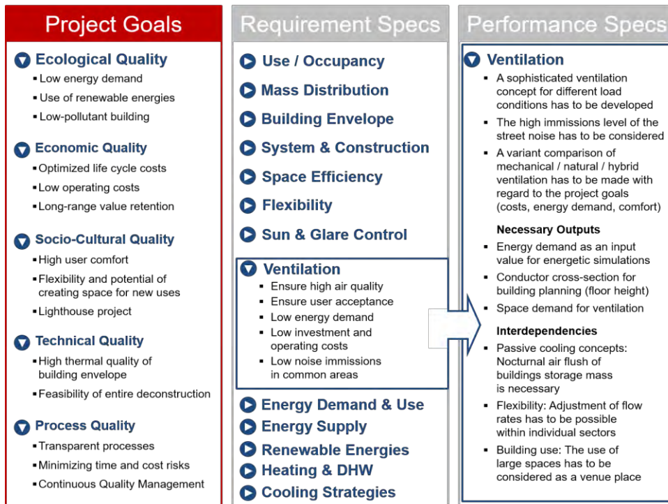
Figure 5: Requirement specs define requests - Performance specs determine related steps for a successful realisation
