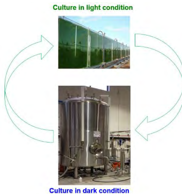
Figure 3: A model system for light-dark recirculate culture
