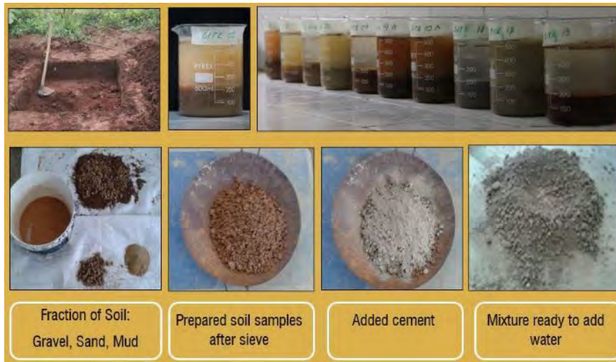
Figure 1: Borrowed soil samples from each site were tested in laboratory and develop the soil up to required level of construction
