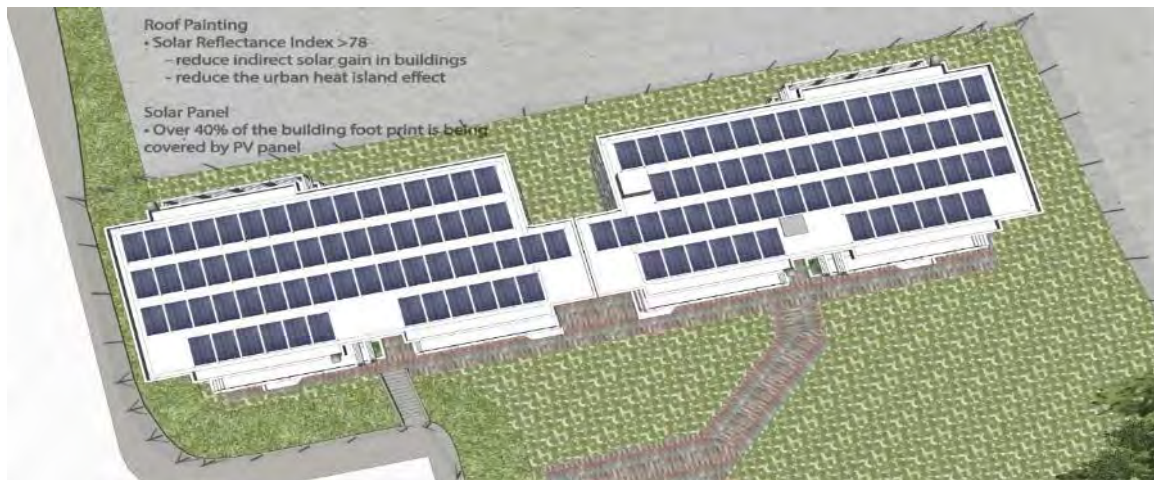
Figure 11: Photovoltaic system installed on the roof of Block A and Block B.
