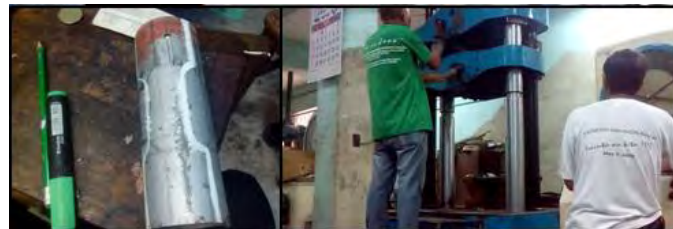
Figure 9: Tensile test (right) on the sample (left)
