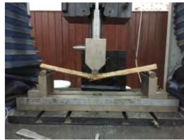
Figure 1116: Bending test -longitudinal modulus of elasticity (Author)
