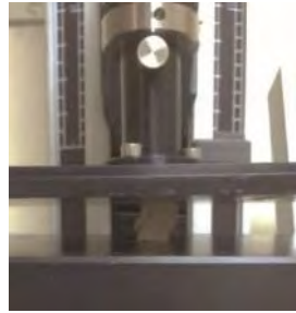
Figure 1114: Compression test perpendicular to fibers (Author)
