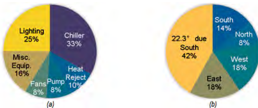
Figure 3: The percentage of year-round (a) Power consumption and (b) PV power production
