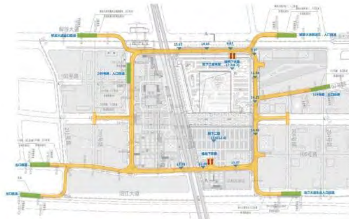
Figure 6: Wuhan CTF Finance Centre: underground vehicular loop road with community parking at B2&3
