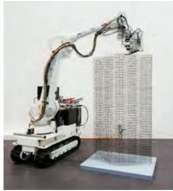
Figure 1: Robotically fabricated metal Mesh Mould structure
