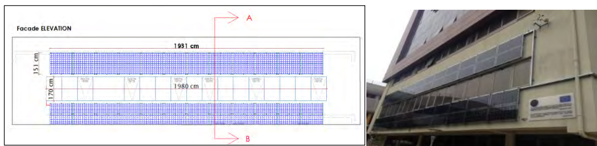
Figure 1: A schematic and picture of the BIPV system installed
