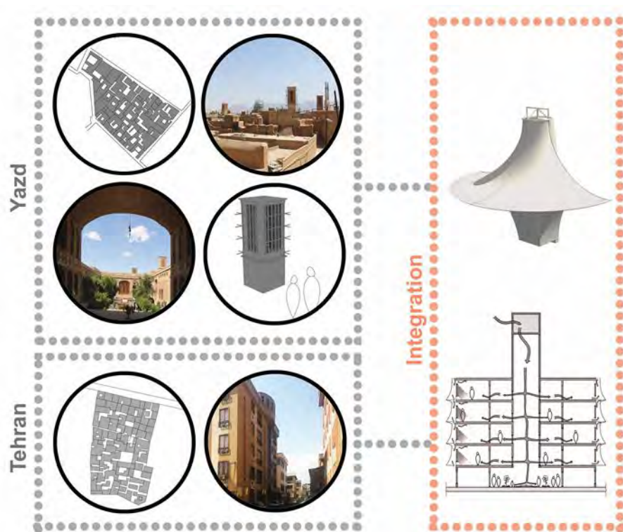
Figure 1: Framework diagram: Existing urban context and vernacular windcatchers of Yazd (upper left) compared with dense modern urban context of Tehran (bottom left) informing new strategies for integration of windcatcher concepts through tensile fabric techniques
