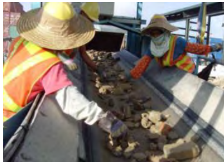
Figure 6: Manual picking unwanted constituents in C&D Waste at sorting facility in Tseung Kwan O Area 137
