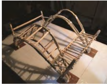
Figure 13: Adding the space truss bracings using friction connections (Author)
