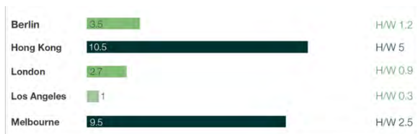
Figure 5: Calculated maximum change in air temperature due to green facades in correlation with height-to-width ratio of street canyons
