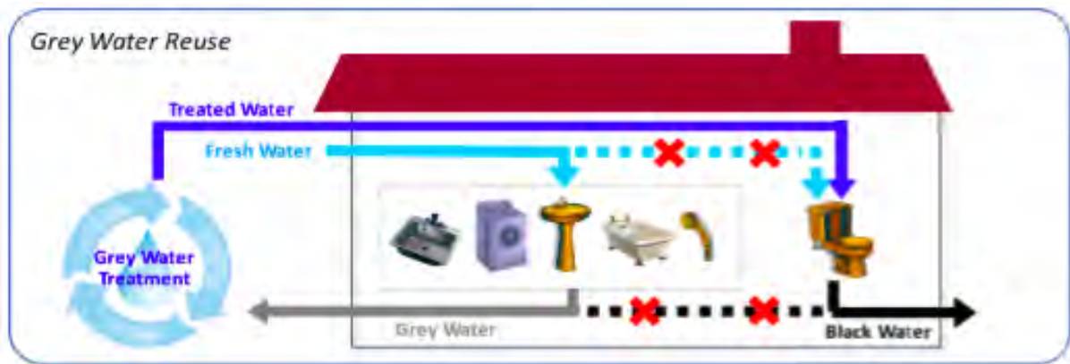
Figure 2: Schematic diagram for grey water recycling
