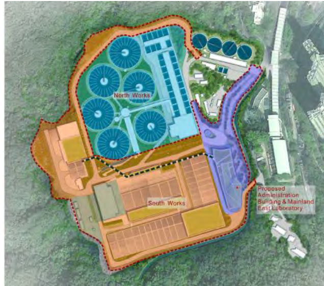
Figure 1: Layout Plan of STWTW with Reprovisioned Administration Building and South Works Treatment Process Precinct
