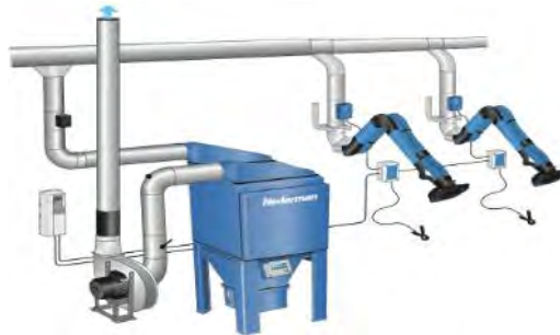
Figure 5: Welding fume collector
