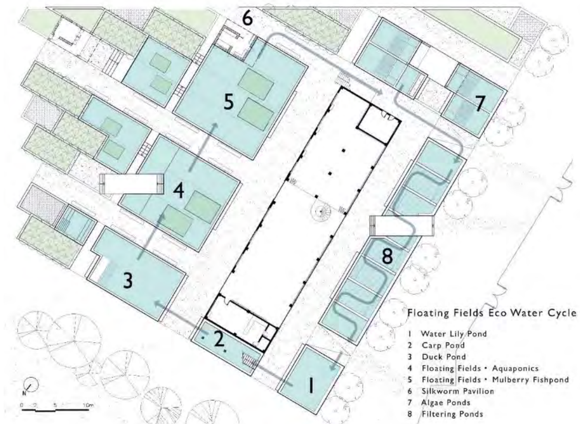
Figure 2: Eco-water cycle plan diagram showing complete cycle from 1 to 8.
